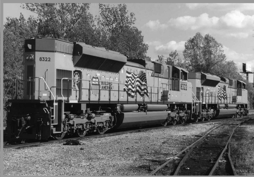
A pair of freshly assembled and painted EMD locomotives are ready for delivery to Union Pacific. These yellow and gray monsters, UP SD70ACes 8322 and 8356 were caught at P&I junction in Paducah, KY on April 27, 2005. These units were probably assembled from kits as shown above. Photo by Wallace Henderson
