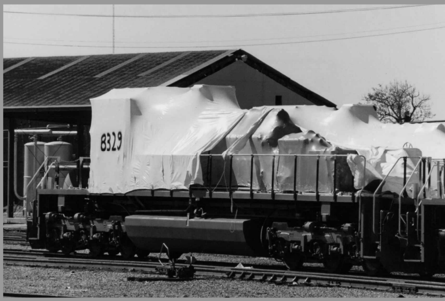
A shrink-wrapped chassis and internal parts - prime mover, generator, etc. - is at the NRE (VMV) backlot. From all that we have been able to gather these are SD70ACe locomotive kits that are being assembled and finished for delivery to Union Pacific. photo by Wallace
